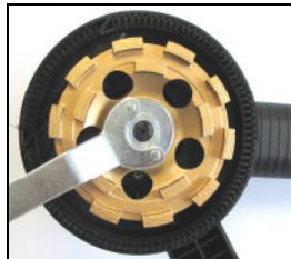
Pay attention that the collar of the clamping nut faces away from the machine, as shown in the figure.
