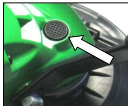
Actuate the spindle stop and keep it pressed.
