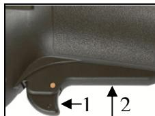
Switching-on: push the lock-off button forward (1) and then the on/off switch down (2)
